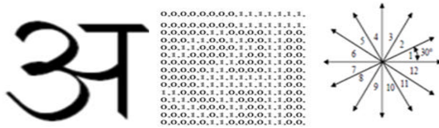
Fig. 2: Binary representation of character ‘A’ and directional feature extraction
