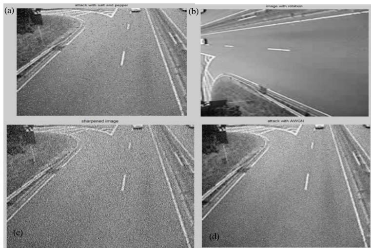
Fig. 8: Attacks added to embedded image samples: a) Salt and pepper noise; b) Rotation; c) Sharpening noise; d) AWGN
