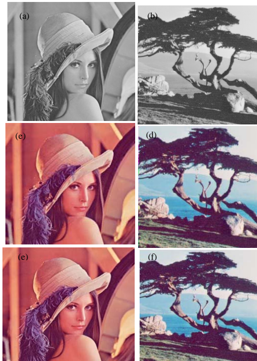
Fig. 7: a, b) The original images of Lenna and Pine; c, d) The composite images of Lenna and Pine and e, f) The retrieved images of Lenna and Pine for Isosceles Triangle approach
