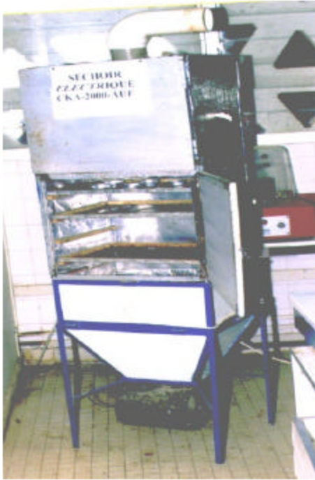
Fig. 1: Forced convection dryer (Haq, 2000) used in the study
