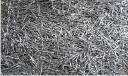
Fig. 4: Steel fiber used in the experiment
