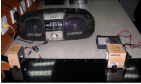
Fig. 8: The experimental setup to test the largest distance that the LED
