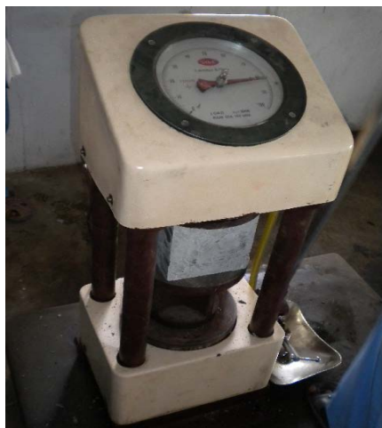
Fig. 3: Testing of beam cubes
