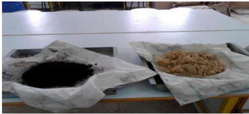
Fig. 2: Treated pumice and limestone cubes after crushing
