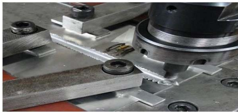
Fig. 6: FSW experimental with thermocouple (Wang et al. , 2015)
