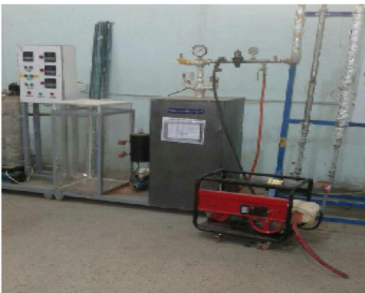
Fig. 4: The modified steam engine and steam generator setup for test
