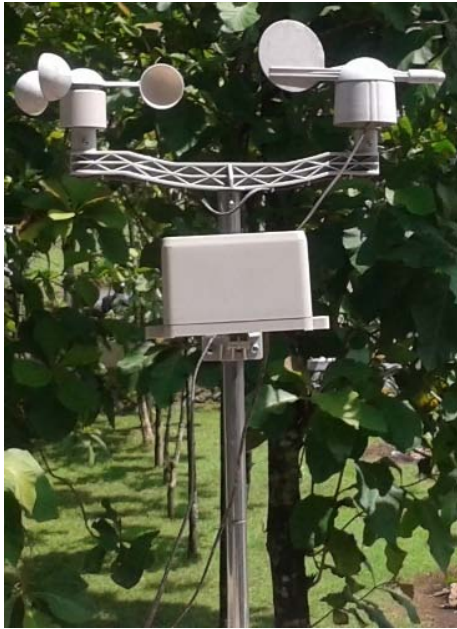
Fig. 5: Anemometer and wind vane to measure velocity and wind direction
