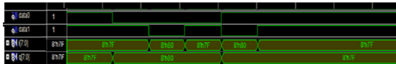
Fig. 7: Timing simulation of The QPSK modulator at random values
