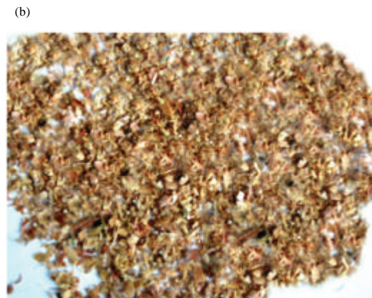
Fig. 6: a) Wood chip coarse fibre and b) Sawdust coarse fibre
