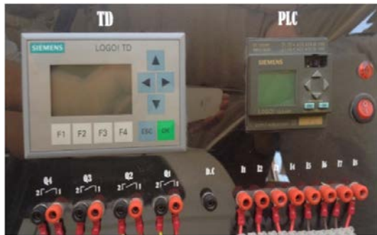
Fig. 11: Main part of the controlling system
