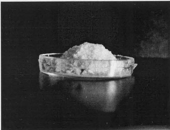
Fig. 2: Freeze-dried products from 1:10 (meat/water ratio) whole spent hen breast meat suspension
