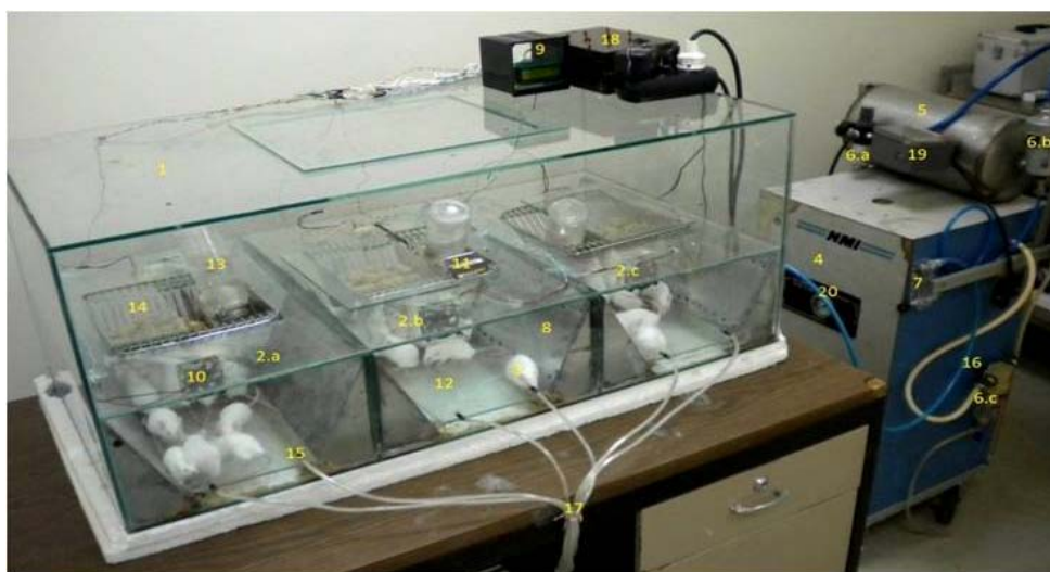
Fig. 1: Appearance of DE model. 1: DEC (Dry Eye Cabin), 2 (a-c): EAD (Experimental Animal Division), 3: The subjects, 4: AC (Air Compressor), 5: AC tube, 6 (a-c): Water separator, 7: Flowmeter, 8: Desiccators' containers, 9: Control board, 10: Fan, 11: Humidity-Temperature monitor, 12: Mobile glass plates, 13: Watering, 14: Feeder, 15: Air inlet holes, 16: Pneumatic pipes, 17: Flexible inhalation hose, 18: Fan switch board, 19: AC pressure monitor, 20: AC pressure gauge
