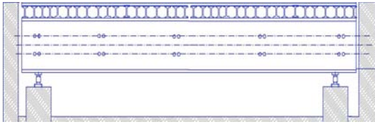
Fig. 2: Motor truck scales NPV 30000 kg
