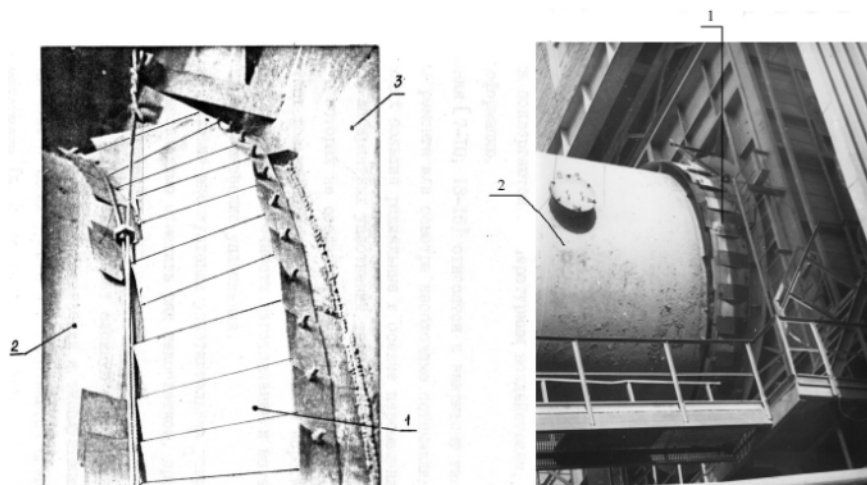
Fig. 1: Sealing of rotary kilns: 1 sealing, 2 oven, 3 fridge
