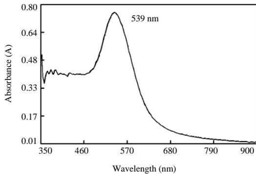
Fig. 5: UV-visible spectrum of gold nanoparticles (D)
