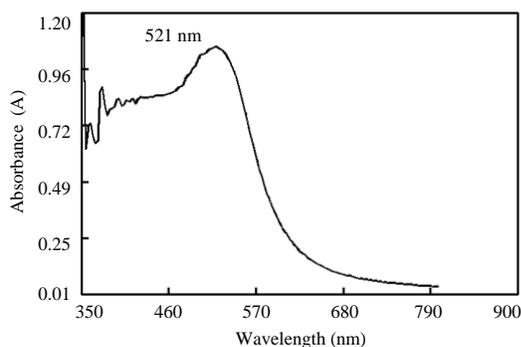
Fig. 8: UV-visible spectrum of citrate stabilized gold nanoparticles
