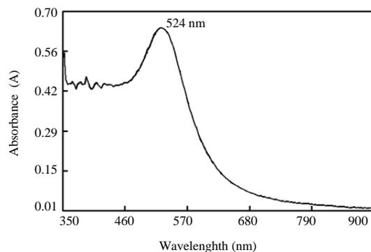
Fig. 3: UV-visible spectrum of gold nanoparticles (B)
