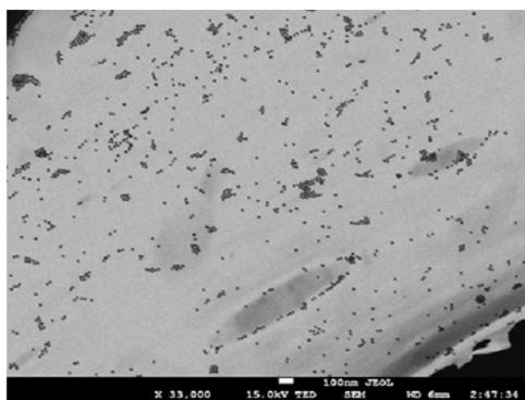
Fig. 9: FESEM micrograph of citrate stabilized gold nanoparticles
