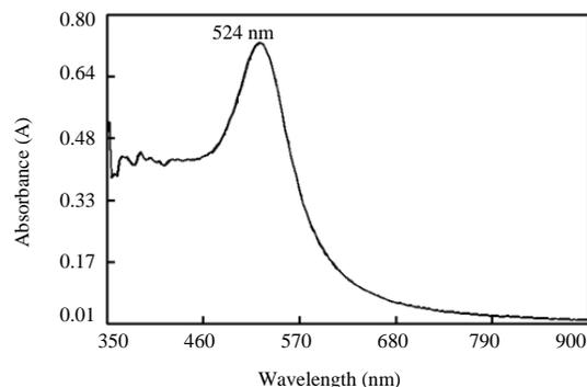
Fig. 2: UV-visible spectrum of gold nanoparticles (A)
