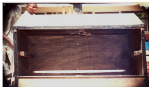
Fig. 3: Forced airflow cabinet dryer used in drying differently salted O. niloticus
