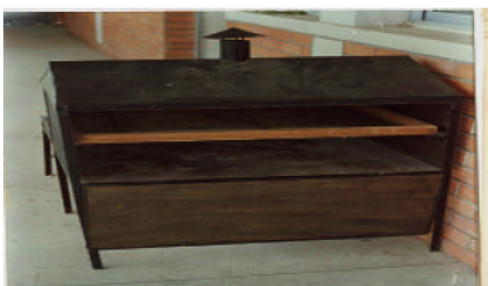
Fig. 2: Natural airflow cabinet dryer (nacd) used in drying differently salted O. niloticus
