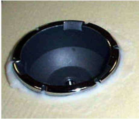
Fig. 6: PU-bloc with the cemented C-MIC-cup
