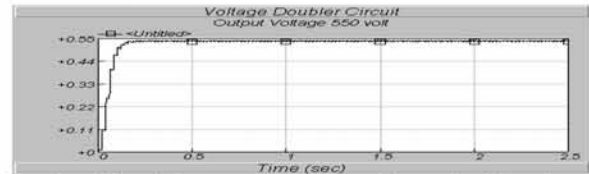
Fig. 9: Simulation result of the voltage doubler circuit by PSCAD
