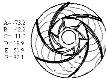
Fig. 9: The static pressure (KPa) contours in impeller when handling the oil ( \nu=43 \times 10^{-6} \text{ m}^2/\text{s} )
