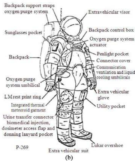
Fig. 1: (a) Apollo 11 A7L space suit (b) diagram showing component parts of A7L space suit
