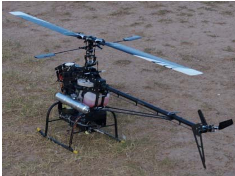
Fig. 2: Velocity 90-based medium size unmanned disaster relief helicopter under development at Aerial Robotics Lab., NUST, Pakistan.
