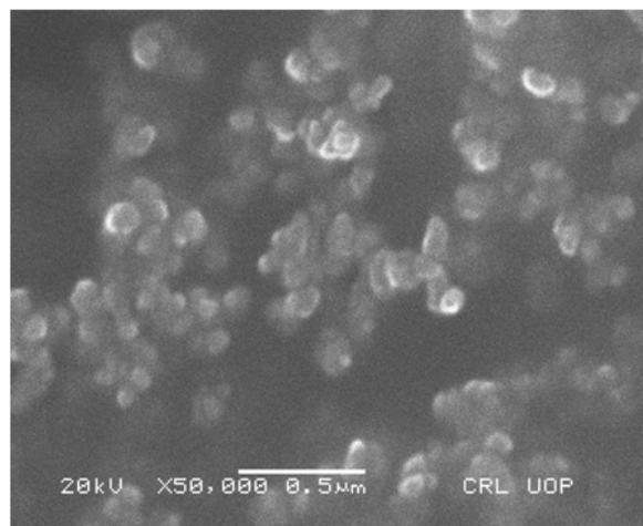
Fig. 5: SEM image of synthesized silver nanoparticles.
