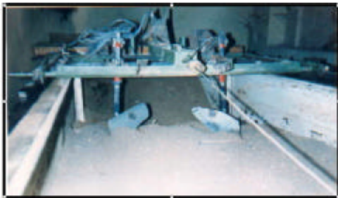
Fig. 2: Small-scale models assembled on tool carriage
