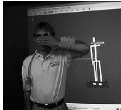
Fig. 6: Tracking of the arm using three MARG sensors (Bachmann)
