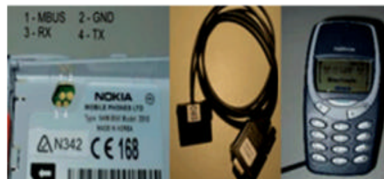
Fig. 4: F-bus pins, f-bus connector, Nokia 3310 mobile
