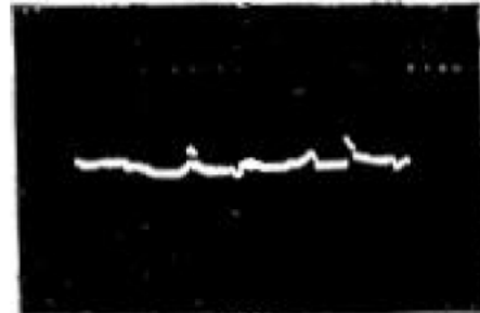
Fig. 15: Coil voltage (recorde between the main and the auxiliary brushes glued together on top by an adjoining flexible bridge with A_w = 2.1 mm; b_g = 0.40 mm; I_a = 12A )
