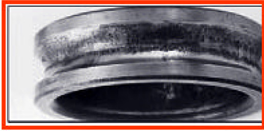
Fig. 1: Chipping on the interior ring of a ball-bearing deeps-groove
