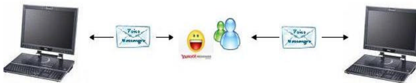
Fig. 3: Software (Yahoo/MSN messenger for Voice Chat. etc.) a microphone, speakers, a sound card and an Internet connection
