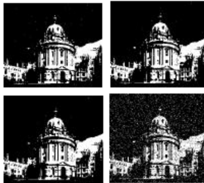
Fig. 5: Performance study of a communication system in Rayleigh channels (SNR = 15dB). (a) Transmitted image, (b) Received image in 2-PSK modulation techniques, (c) Received image in QPSK and 4-QAM modulation techniques and (d) Received image in 16-QAM modulation techniques
