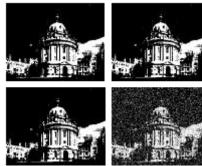
Fig. 7: Performance Study of a communication system in Rician channels (SNR = 15dB). (a) Transmitted image, (b) Received image in 2-PSK modulation techniques, (c) Received image in QPSK and 4-QAM modulation techniques and (d) Received image in 16-QAM modulation techniques
