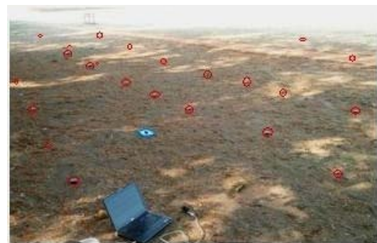
Fig. 11: Deployment of 24 IRIS nodes (circled in red) and mobile sink (circled in blue)
