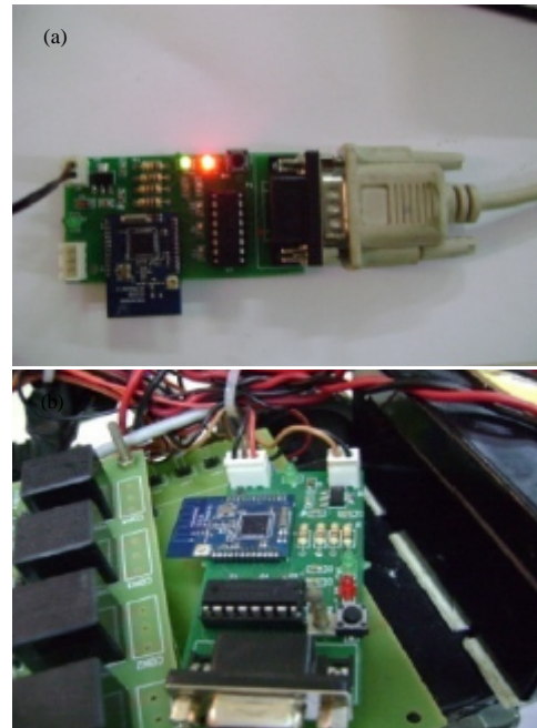
Fig. 4: Zig bee module: a) Interface RS232 with Zig bee at PC; b) Interface Zig bee at robot side
