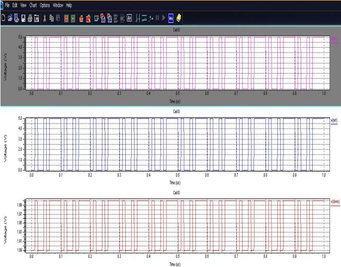
Fig. 4: Timing diagram of DPF up conversion
