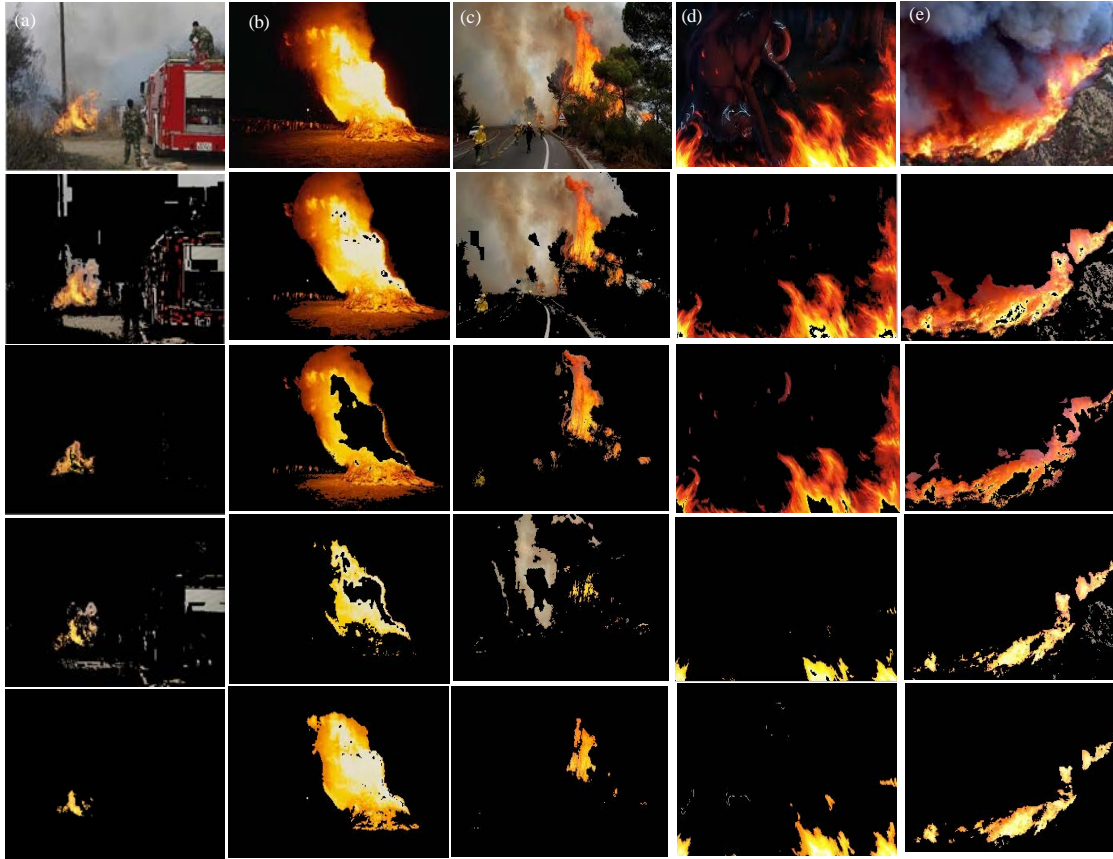
Fig. 13: Result of fire pixel segmentation in various color spaces; a) RGB; b) YUV; c) CIE L*a*b* and d) YCbCr
