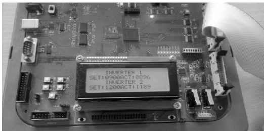
Fig. 9: Set Speed using FPGA
