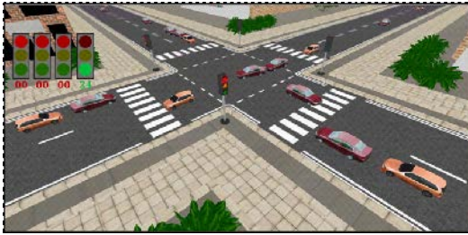
Fig. 4: Screen shoot of the HIL system with traffic light simulation and countdown
