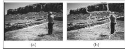
Fig. 3: Segmentation of the image: a) Original image; b) Using normalized cuts segmentation
