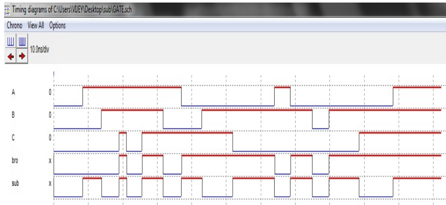
Fig. 12: The 8T 1-bit full subtractor pulse waveform
