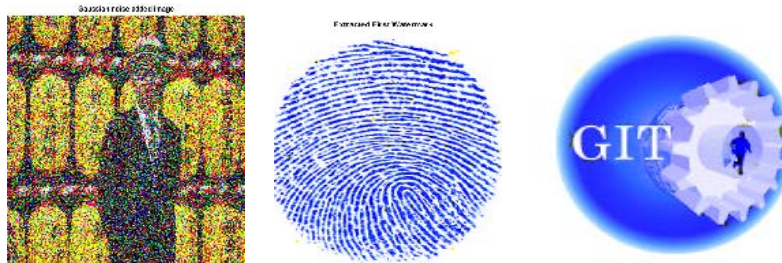
Fig. 15: a) Gaussian Noise added watermarked image; b) Extracted primary watermark with NC = 0.9980 ; c) Extracted secondary Watermark with NC = 0.9701
