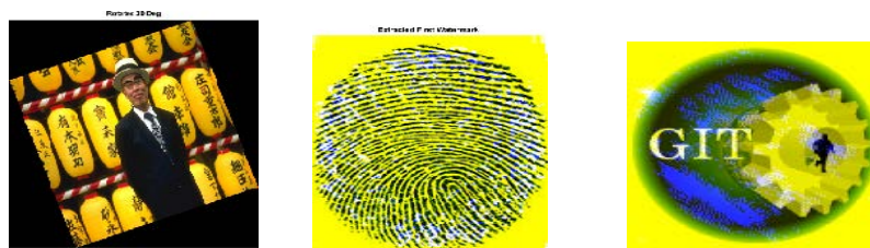
Fig. 17: a) Rotated watermarked image at 20; b) Extracted primary watermark with NC = 0.7888 ; c) Extracted secondary watermark with NC = 0.8188
