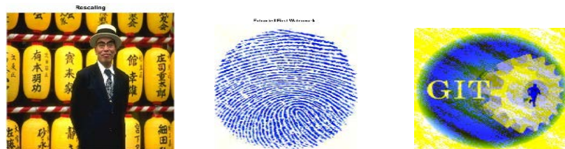
Fig. 18: a) Rescaled by [384 \ 384] : 0.75 ; b) Extracted primary watermark with NC = 0.9997 ; c) Extracted secondary Watermark with NC = 0.8778
