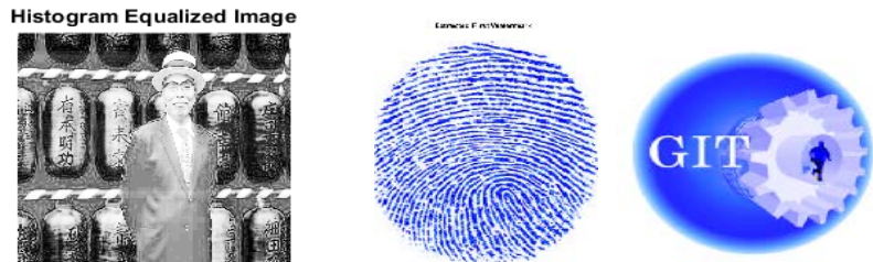
Fig. 8: a) Histogram equalized watermarked image; b) Extracted primary watermark with NC = 0.9987 ; c) Extracted secondary watermark with NC = 0.9707
