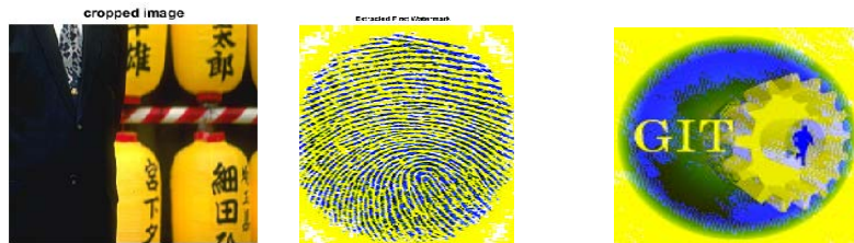
Fig. 15: a) Gaussian Noise added watermarked image; b) Extracted primary watermark with NC = 0.9980 ; c) Extracted secondary Watermark with NC = 0.9701
