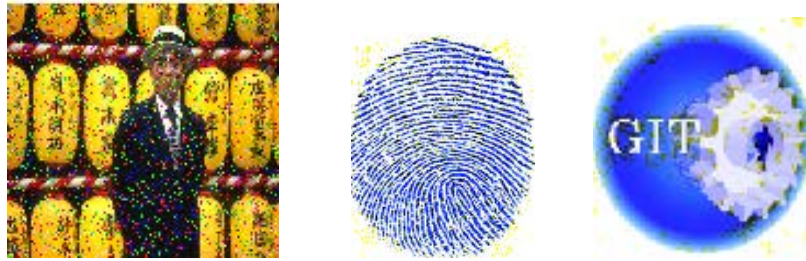
Fig. 7: a) Salt and pepper noised image with s = 0.1 ; b) Extracted primary watermark with NC = 0.9849 ; c) Extracted watermark with NC = 0.9585
