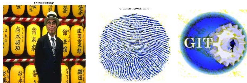
Fig. 13: a)Edge Sharpened Watermarked Image; b)Extracted primary watermark with NC = 0.9875; c) Extracted secondary Watermark with NC = 0.9497
