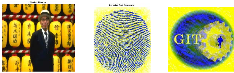
Fig.12: a)Median filtered Watermarked Image; b)Extracted primary watermark with NC = 0.9437 ; c) Extracted secondary Watermark with NC = 0.8122
