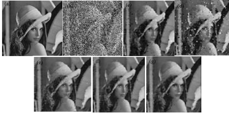
Fig. 2: Restored images: a) Original image; b) 50% noisy image; c) Simple median filter; d) Single threshold algorithm; e) Dual threshold algorithm; f) Condition based algorithm and g) Proposed algorithm
