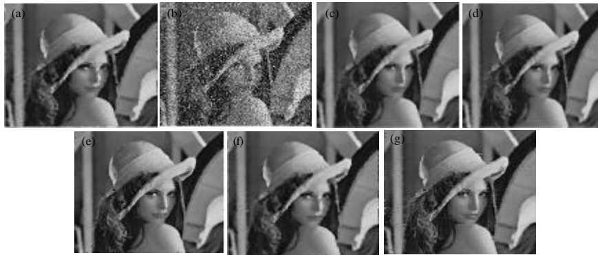
Fig. 3: Restored images: a) Original image; b) 90% noisy image; c) Simple median filter; d) Single threshold algorithm; e) Dual threshold algorithm; f) Condition based algorithm and g) Proposed algorithm
