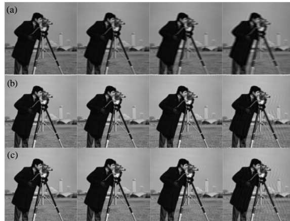
Fig. 3: Restored images obtained from synthesized images with blur lengths L = 8, 12, 18, 21 , respectively by: a) Wiener filter; b) LR method; c) Proposed method
