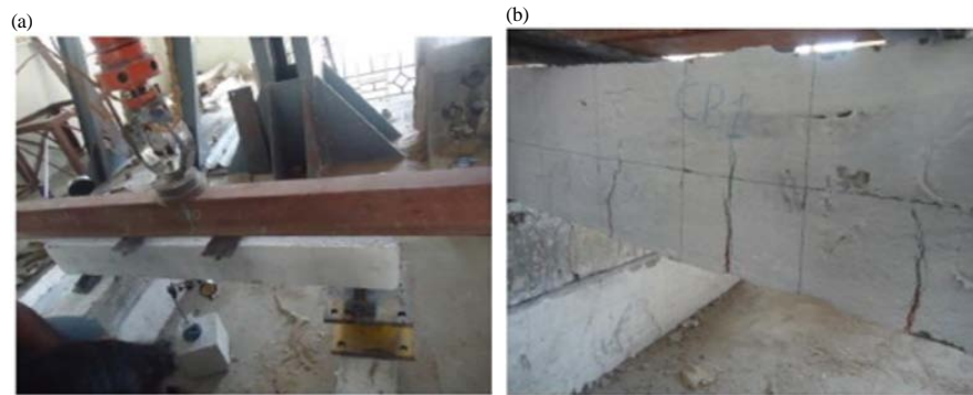
Fig. 4: Control specimen: a) Before loading of control beam and b) After loading of control beam
