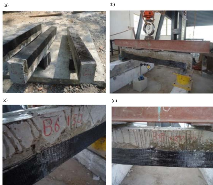
Fig. 5: Retrofitted specimen: a) Retrofitted beam before loading; b) Retrofitted beam GP bonded CFRP; c) Retrofitted beam Iso bonded CFRP and d) Retrofitted beam epoxy bonded CFRP
