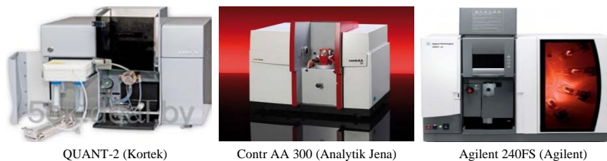
Fig. 3: Russian and German atomic-absorption spectrometers
