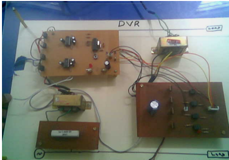
Fig. 12: Laboratory model of DVR system
