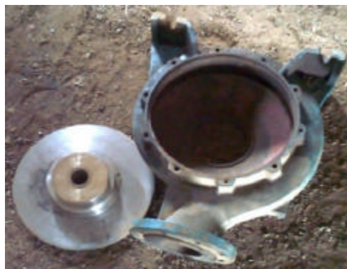
Fig. 7: The turbine housing/casing and conversion plates
