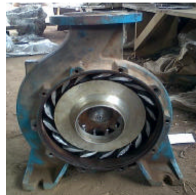
Fig. 15: Front view of turbine assembly without the casing cover
