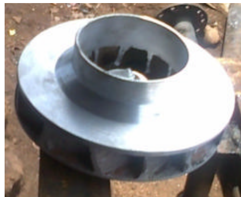
Fig. 6: The finished runner
