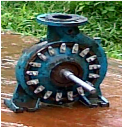
Fig. 16: Back view of turbine assembly
