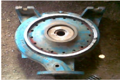
Fig. 8: Back view of the turbine housing
