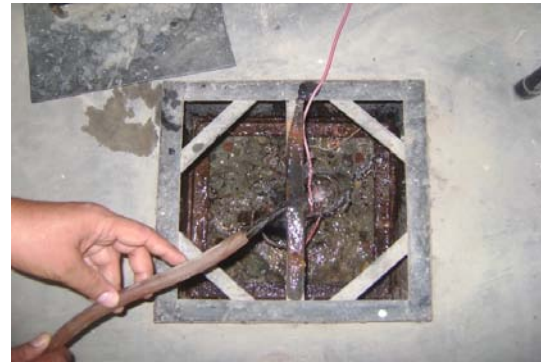
Fig. 4: Watering of electrode point in NIT-Hamirpur HVE laboratory
