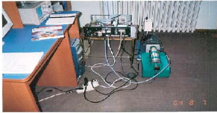
Fig. 13: The photo illustrating switched reluctance motor, DC shunt generator and SR driver circuit set
